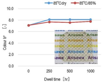
Sample making condition: Pressing at 160°C×60min×3 MPa
