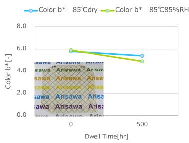
Sample making conditions: Pressing at 160°C×60min×3 MPa
